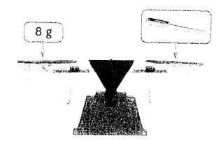
Use mass weights on one side of the balance and the object on the other side. When the sides are balanced, the objects have the same mass.
